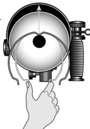
**Warning:** Never operate light without protective screen installed.
